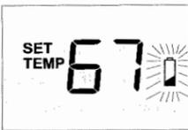
**Note:** The thermostat will still keep the current Set Temperature and Filter run time in memory until new batteries are installed. After confirming that new batteries have been inserted, the thermostat will return to normal operating.
