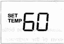
The display will return to the normal room temperature after the keys have been released for 5 seconds.
