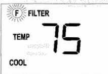
After changing or cleaning the system filter, press and hold the Filter key for 3 seconds. The display will blink, and the counter will be reset to zero.
