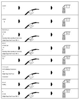
NOTE: Do not connect a "Common" wire (sometimes labeled "C") to any terminal on this thermostat. Tape up the wire and do not use. This wire provides electricity to non-battery powered thermostats.
